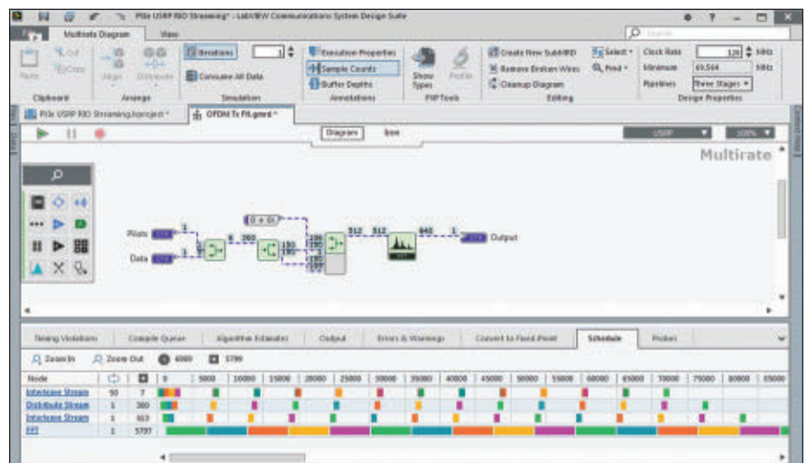
▲ Fig. 3 The LabVIEW Communications multirate diagram makes it easier to convert algorithms from floating-point to fixed-point implementations.
