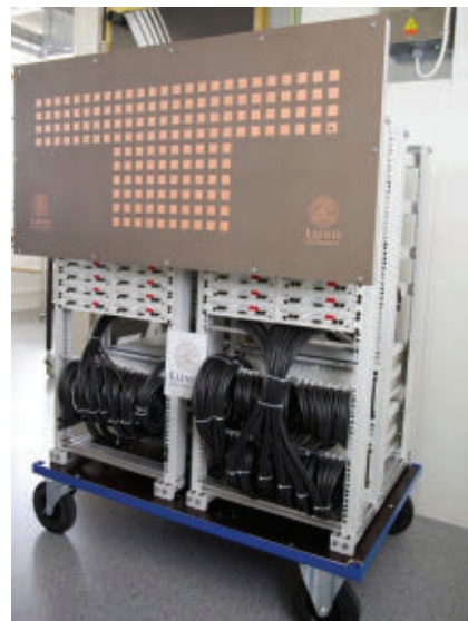
▲ Fig. 8 Massive MIMO prototype developed by Lund University.
