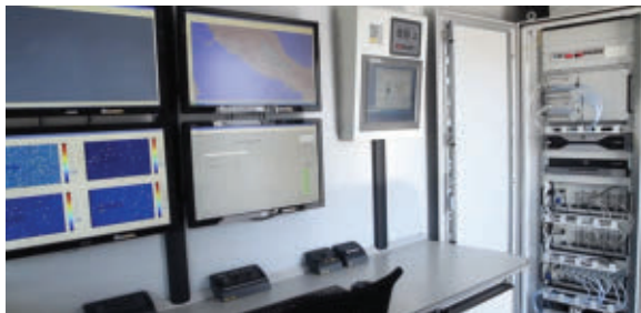
▲ Fig. 9 Complex systems such as this passive radar are designed and deployed with PXI instruments embedded into the final system.
